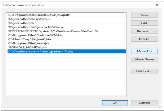
Now to set GRADLE\_HOME under System Variables select click on new and add new system variable: Variable name= "GRADLE\_HOME" and Variable value=<"path where gradle is located"> for example = < C:\Gradle >
